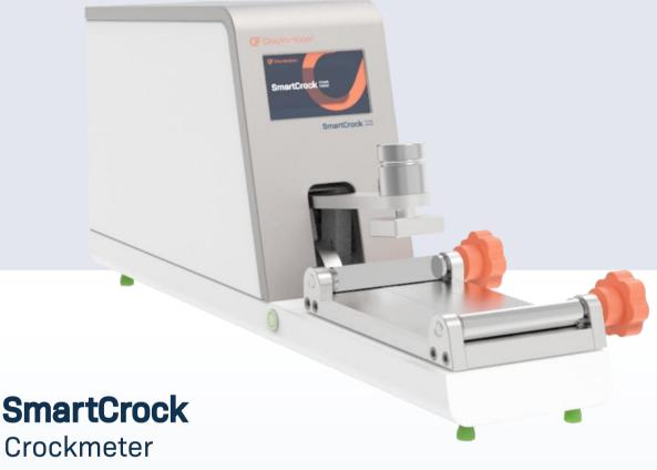
SmartCrock Crockmeter is used to test the color fastness of textiles or leather to dry or wet rubbing. In the test, a standard white rubbing cloth is rubbed repeatedly against a sample at a certain speed. After the test, you can rate color fastness by comparing the color depth of the friction cloth with the standard grey card. They do this under a standard light.
