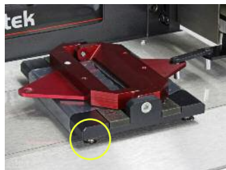
Lift pins retract into the instrument and the sled is placed in the same position each time
