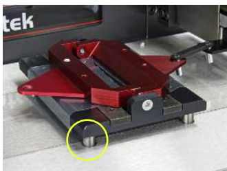
Sled is positioned on lift pins
