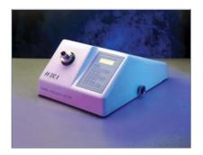
drawn through the sample by a vacuum pump supplied with the instrument. Electronic sensors measure both the airflow and the air pressure, from which the fibre diameter is automatically calculated.
